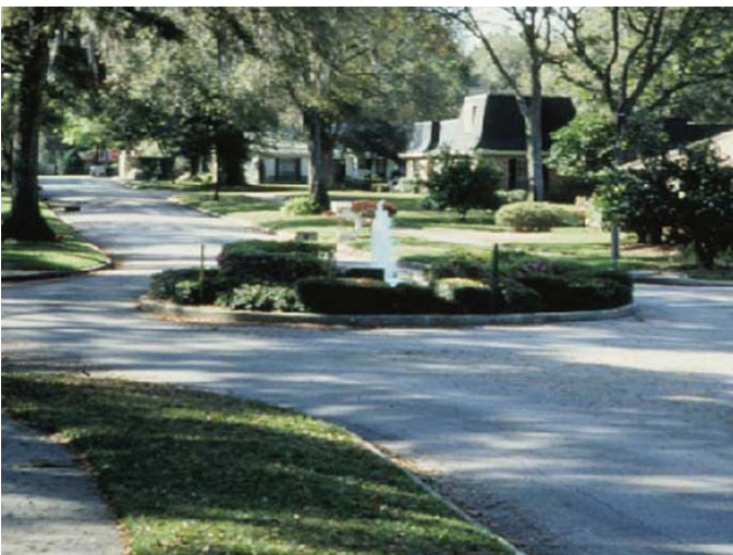
A properly designed roundabout slows intersection traffic, but still allows buses, emergency vehicles and trucks to pass.
