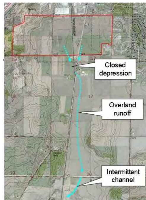
Figure 6-9. Surface water drainage south of the North Stoner Prairie Neighborhood.
